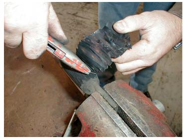
**Step 3.** Remove rubber from O.D. of cross pin. The cross pin must be completely free of all rubber . When using the method pictured above use <a href="Extreme Caution"><u>Extreme Caution</u></a>. Install cross pin noting the correct offset direction noted from step 2.
