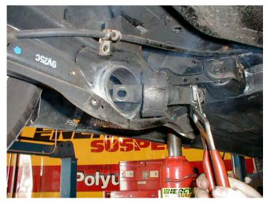
**Step 2.** Important Notes: Do not remove O.E. Outer metal shell. This shell is tapered on O.D.. Make note of which direction the cross pin is installed, this pin is offset! **Bushing / pin removal.** 1. Remove rubber bushing and / or pin from O.E. shell. (One example method to remove rubber bushing from O.E. shell is to use a hacksaw blade and cut bushing out. Note: All rubber must be removed from shell and clean for installation of new bushing.
