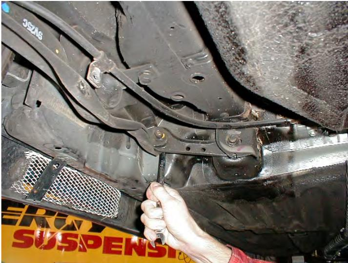
**Step 1.** Remove outer compensator arm bolt only. Remove two mounting bolts at cross pin, and parking brake cable retainer. At this time it is your discretion to remove complete trailing arm from vehicle to facilitate easier removal and installation of new polyurethane bushing or you may pull front of trailing arm downward.
