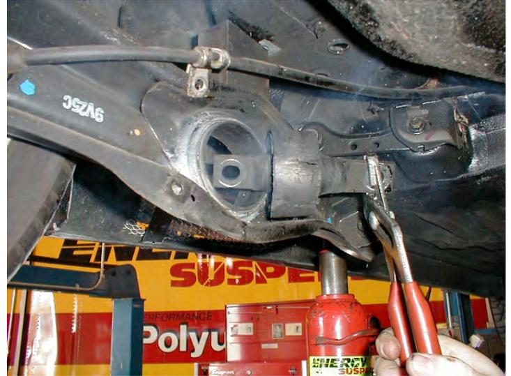
**Step 2.** Important Notes: Do not remove O.E. Outer metal shell. This shell is tapered on O.D.. Make note of which direction the cross pin is installed, this pin is offset! **Bushing / pin removal.** 1. Remove rubber bushing and / or pin from O.E. shell. (One example method to remove rubber bushing from O.E. shell is to use a hacksaw blade and cut bushing out. Note: All rubber must be removed from shell and clean for installation of new bushing .
