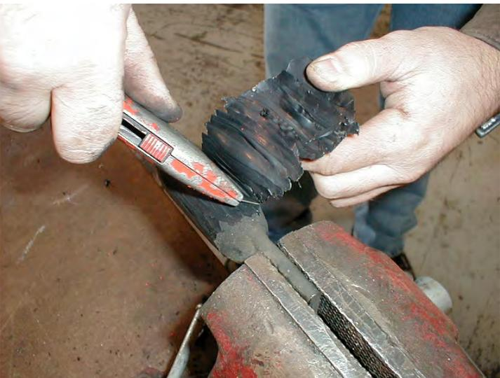
**Step 3.** Remove rubber from O.D. of cross pin. The cross pin must be completely free of all rubber . When using the method pictured above use Extreme Caution. Install cross pin noting the correct offset direction noted from step 2.
