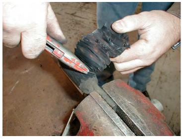
**Step 3.** Remove rubber from O.D. of cross pin. The cross pin must be completely free of all rubber . When using the method pictured above use <a href="Extreme Caution"><u>Extreme Caution</u></a>. Install cross pin noting the correct offset direction noted from step 2.
