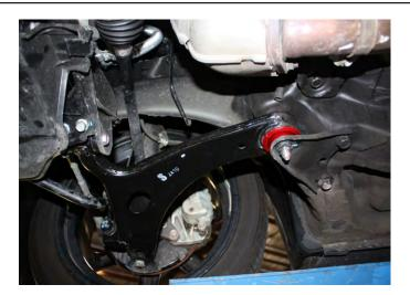
Install the bushing with p/n 03P03529 up. Only grease the leading edge to help get the bushing started. Do not grease the I.D. when installing the inner sleeve.
