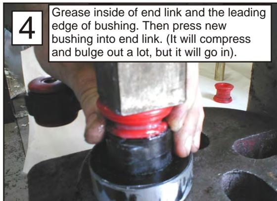
Grease inside of end link and the leading edge of bushing. Then press new bushing into end link. (It will compress and bulge out a lot, but it will go in).
