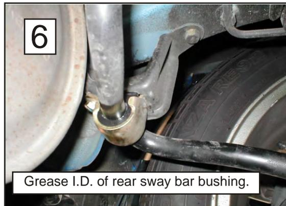
Grease I.D. of rear sway bar bushing.
