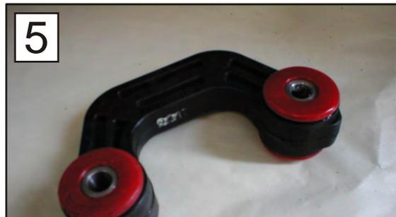
Grease O.D. of metal sleeves and press into I.D. of new bushings.
