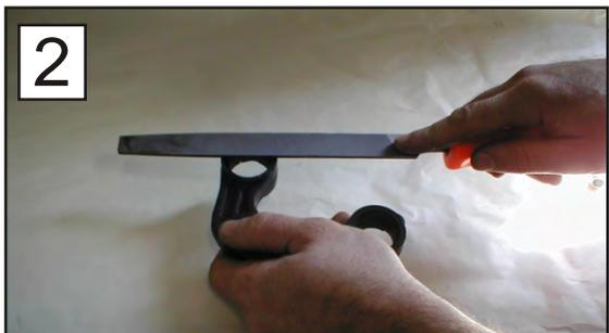
Using a flat file, remove all sharp edges from outer edges of end link.
