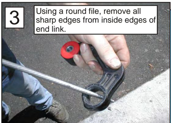
Using a round file, remove all sharp edges from inside edges of end link.
