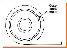
**Note:** When a sleeve is not used, apply a light coat of grease to the original shoulder bolt. **Remember:** Most spring eyes have an outer metal shell. Some shackles are this way as well. The outer
