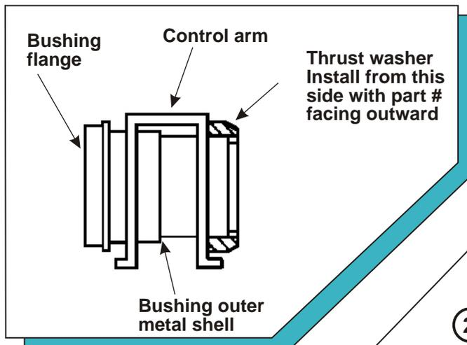
The thrust washers are designed to prevent the control arm from walking side-to-side by accepting side load pressure created during hard cornering. Most kits contain more than one part #. It is very important to install them at the correct location. **See illustration for your set #.**
