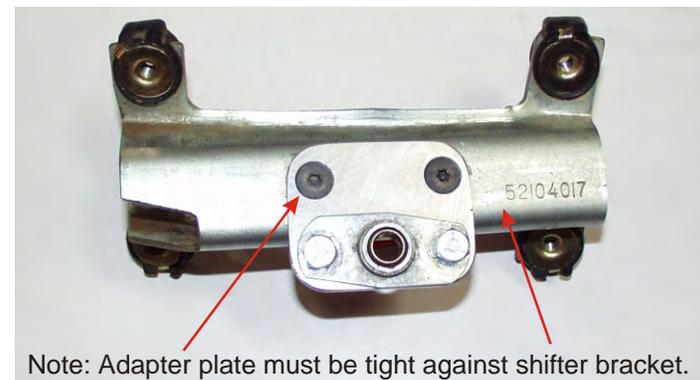
Note: Adapter plate must be tight against shifter bracket.
