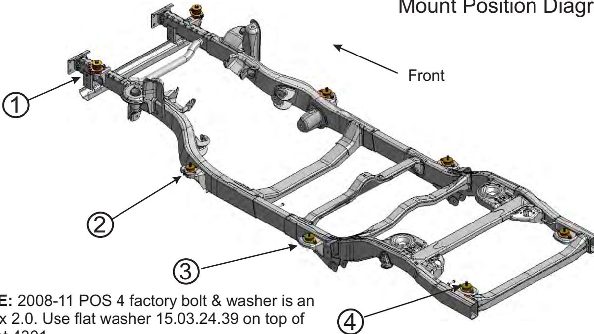
**NOTE:** 2008-11 POS 4 factory bolt & washer is an M14 x 2.0. Use flat washer 15.03.24.39 on top of mount 4301.
