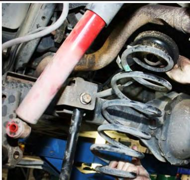
Slowly lower the jacks under the rear axle, allowing the axle to droop. Be careful to not put tension on the brake line. Remove the coil spring and stock rubber isolator from both sides of the vehicle. Mark each coil spring to indicate the driver side and passenger side for reinstallation.
