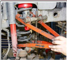
Install the coil springs on their designated sides of the vehicle. A spring compressor may be needed to ease the installation of the spring. Lower the vehicle to ride height. Reconnect the endlinks, lower shock mount, and ABS wires and torque bolts to factory specs. It is recommended to have your vehicle aligned after the installation of these parts.
