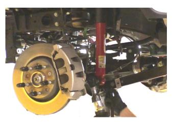
Image 3. Shock Absorber Bolt Removal
