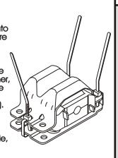
Make sure the tie-wraps are holding firm while releasing the clamp or vise. The metal shells may separate slightly, this is normal. However, excessive separation will prevent mounting botts from reaching through the crossmember allowing the nuts to start on the botts. Cut the ends of the tie-wraps off, being sure not to leave any sharp edges.
