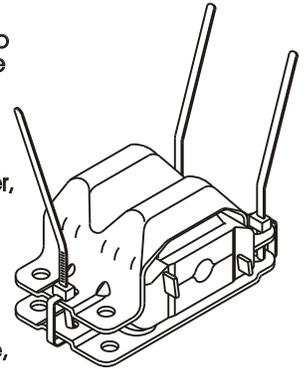
Make sure the tie-wraps are holding firm while releasing the clamp or vise. The metal shells may separate slightly, this is normal. However, excessive separation will prevent mounting bolts from reaching through the crossmember allowing the nuts to start on the bolts. Cut the ends of the tie-wraps off, being sure not to leave any sharp edges.
