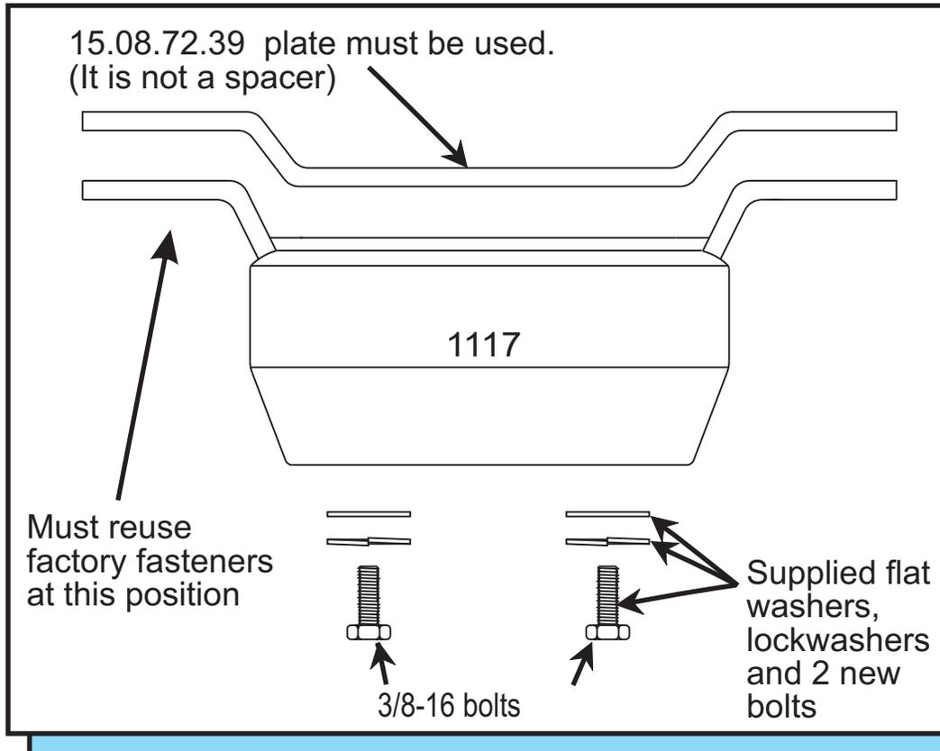
Tighten all fasteners to factory specifications
