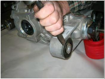
2. You will need to press the old bushings out. Using one of these process (See Picture Below)
