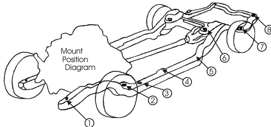
When all mounts and hardware are installed, torque all bolts to factory specifications.
