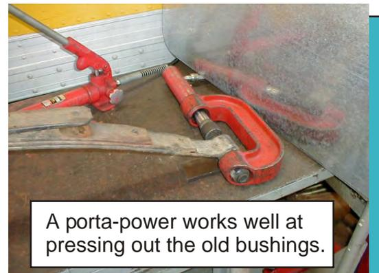
When installing Urethane bushings, apply grease as instructed: Remove the original rubber and outer shell (when used) clean I.D. of the spring eyes and frame brackets of any old rubber or rust with sand paper. Apply a light coat of grease to the eyes of both spring and frame brackets. Apply a light coat to the I.D., O.D. and flange of the bushings. (all surfaces that contact metal) Apply a light coat of grease to the O.D. of the sleeves.)
