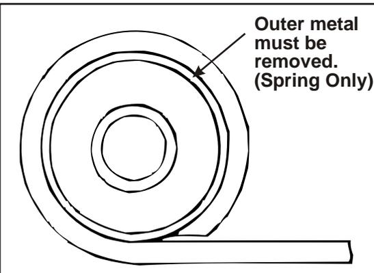
**Remember:** Most spring eyes have an outer metal shell. The outer shell must be removed. A tool rental store will have a Porta-power to press out the shells from the spring eyes.
