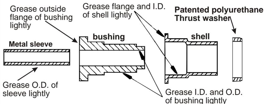
The thrust washers are designed to prevent the control arm from walking side-to-side by accepting side load pressure created during hard cornering. Most kits contain more than one part #. It is very important to install them at the correct location.
