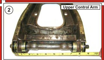
With the end cap washers removed, measure the outside width of shell to shell before pressing out old bushings. At this relaxed state the measurement is approximately 8-1/4" ± 1/16"
