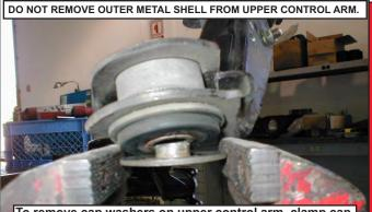
To remove cap washers on upper control arm, clamp cap washer in vice and wiggle arm back and forth. Inner sleeve is not bonded, use spray lube to help press it out.
