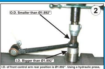
I.D. of front control arm rear position is Ø1.892". Using a hydraulic press, properly support control arm and slowly push out the rubber bushing with bonded outer metal casing. Remove all sharp edges from I.D. Apply grease to all metal parts that will contact the new polyurethane bushings.
