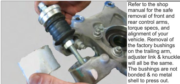
Refer to the shop manual for the safe removal of front and rear control arms, torque specs, and alignment of your vehicle. Removal of the factory bushings on the trailing arm, adjuster link & knuckle will all be the same. The bushings are not bonded & no metal shell to press out.
