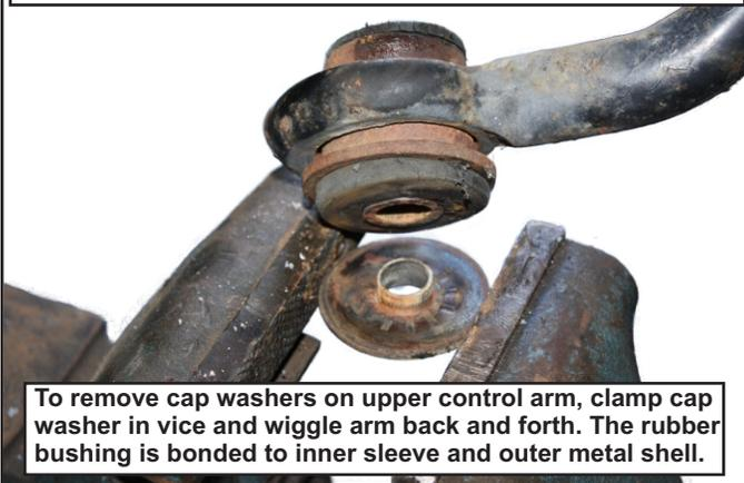
To remove cap washers on upper control arm, clamp cap washer in vice and wiggle arm back and forth. The rubber bushing is bonded to inner sleeve and outer metal shell.
