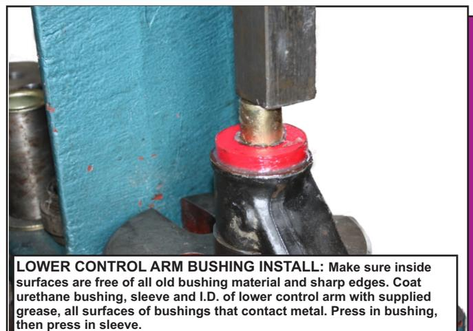
**LOWER CONTROL ARM BUSHING INSTALL:** Make sure inside surfaces are free of all old bushing material and sharp edges. Coat urethane bushing, sleeve and I.D. of lower control arm with supplied grease, all surfaces of bushings that contact metal. Press in bushing, then press in sleeve.
