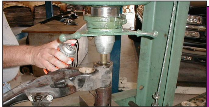
**LOWER CONTROL ARM BUSHING REMOVAL:** There is no outer metal shell to press out. The rubber bushings are bonded to the inner sleeve, but not the control arm. Press the bushing/sleeve out as a unit. Use spray lube to help remove the old rubber bushings from the lower control arms.
