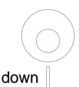
Bushings must be installed with offset hole down and centered in the 6 o'clock position.
