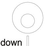
Bushings must be installed with offset hole down and centered in the 6 o'clock position.
