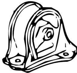
Clean any dirt, grease, and excess rubber flashing that may be present inside the engine mount. **NOTE: IT IS VERY IMPORTANT THAT THE INSIDE OF THE ENGINE MOUNT BE CLEAN AND DRY.**
