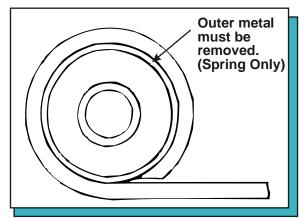
Remember: Most spring eyes have an outer metal shell. The outer shell must be removed. A tool rental store will have a Porta-power to press out the shells from the spring eyes.
