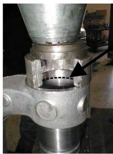
Press the new sleeve in flush to taper
