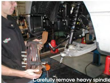
Carefully remove heavy spindle
