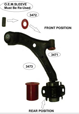
APPLY GREASE TO ALL PARTS THAT CONTACT POLYURETHANE BUSHINGS PRIOR TO INSTALLATION
