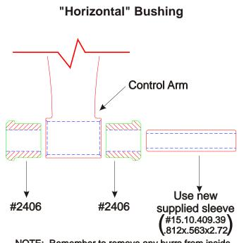
NOTE: Remember to remove any burrs from inside of the control arm to ensure proper operation.
