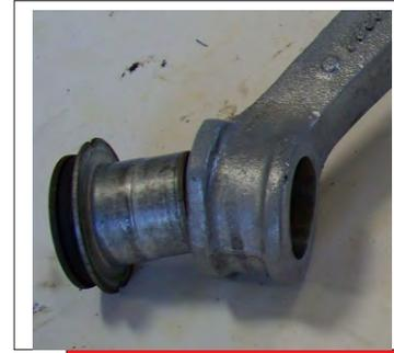
Factory bushing metal shell must be pressed out of upper control arm for Energy Suspension polyurethane bushings to fit properly.
