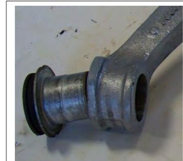
Factory bushing metal shell must be pressed out of upper control arm for Energy Suspension polyurethane bushings to fit properly.
