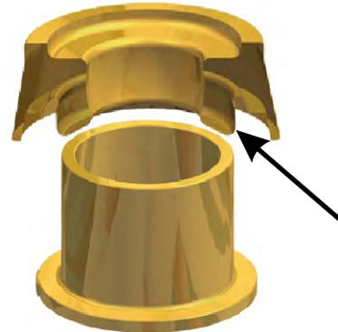
Place the upper vertical bushing #3406 in the metal shell first, this enables you to confirm that the inside edge of the bushing is not pinched at the top of the shell. Neglecting this step could cause the bushing to bind and or eventually tear.
