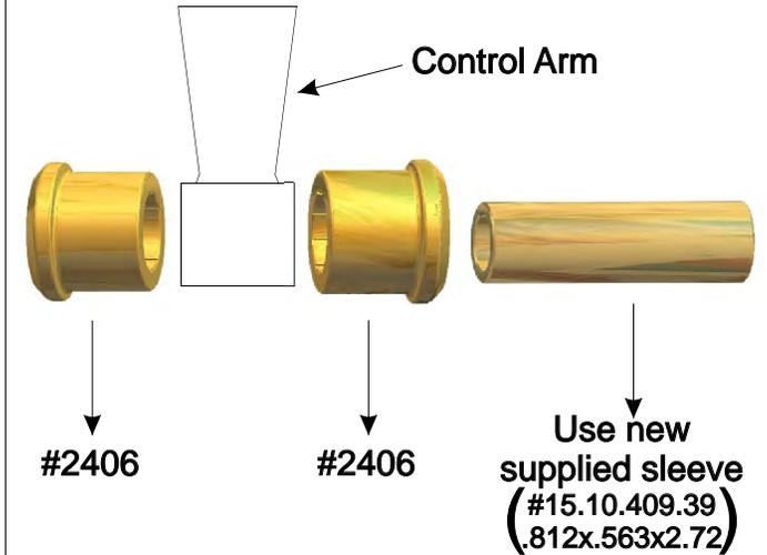
NOTE: Remember to remove any burrs from inside of the control arm to ensure proper operation.
