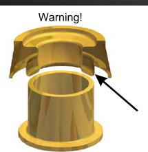
Place the upper vertical bushing #3406 in the metal shell first, this enables you to confirm that the inside edge of the busing is not pinched at the top of the shell. Neglecting this step could cause the bushing to bind and or eventually tear.
