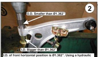
I.D. of front horizontal position is Ø1.362". Using a hydraulic press, properly support control arm and slowly push out the rubber bushing with bonded outer metal casing. Remove all sharp edges from I.D. Apply grease to all metal parts that will contact the new polyurethane bushings.
