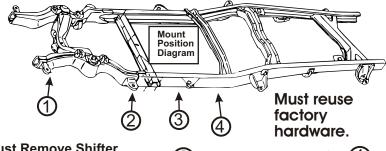
Must Remove Shifter Bracket And Park Brake Clamp From Frame Before Lifting Body
