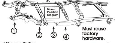
Must Remove Shifter Bracket And Park Brake Clamp From Frame Before Lifting Body
