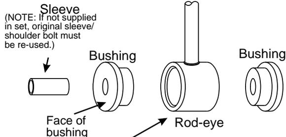
**REMEMBER:** Some O.E. bushings use an outer metal shell, this outer shell must be removed.
