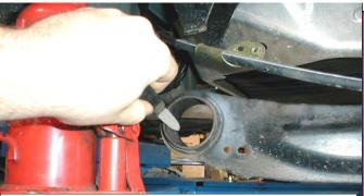
Let metal shell cool before cleaning inside Remove any burrs and sharp edges before applying grease. With both eyes of the trailing arm smooth, clean, and free from sharp metal burrs and any metal shavings.
