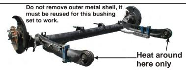
To remove rubber bushing, apply light heat evenly around the outside of the outer metal shell, just enough to brake the bond with the rubber. When you see light smoke coming from the sides of the bushing the bond should be broken. (At no time should there be any flames coming from the rubber, if there are any flames, you need to back off with the heat). Just push the old rubber and inner metal sleeve out. Let the outer metal shell cool off before cleaning the
