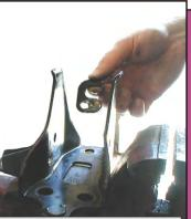
Use a chisel on the inside to break away remainder of tab. Use a file to remove all sharp edges that might cut or rip the new polyurethane bushings.
