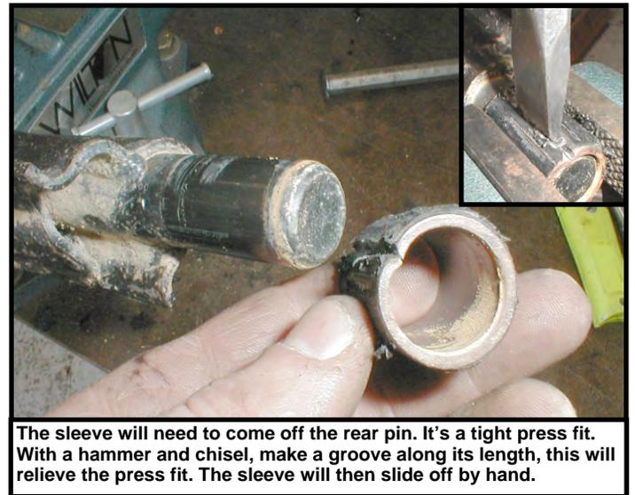
The sleeve will need to come off the rear pin. It's a tight press fit. With a hammer and chisel, make a groove along its length, this will relieve the press fit. The sleeve will then slide off by hand.
