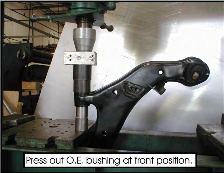
Press out O.E. bushing at front position.
