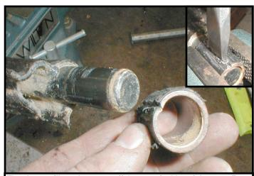
The sleeve will need to come off the rear pin. It's a tight press fit. With a hammer and chisel, make a groove along its length, this will relieve the press fit. The sleeve will then slide off by hand.
