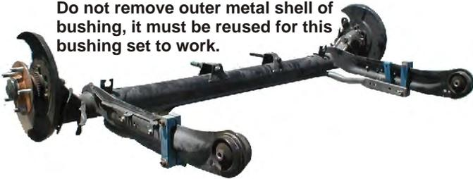
To remove rubber bushing, apply low heat evenly around the outside of the outer metal shell, just enough to break the bond with the rubber. When you see light smoke coming from the sides of the bushing the bond should be broken. At no time should there be any flames coming from the rubber, if there are any flames, you need to back off with the heat. Just push the old rubber and inner metal sleeve out. Let the outer metal shell cool off before cleaning the inside.
