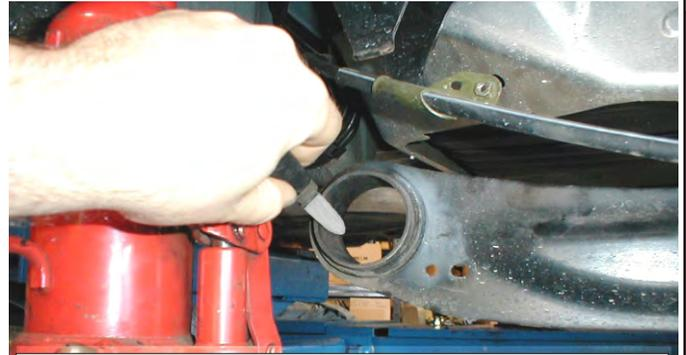
Let metal shell cool before cleaning inside. Remove any burrs and sharp edges before applying grease.
