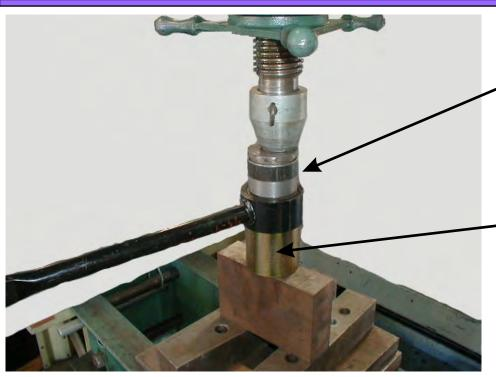
Inside Dia. of tension rod is 2.512" (63.8mm). Push out old bushing with something smaller than 2.512".
