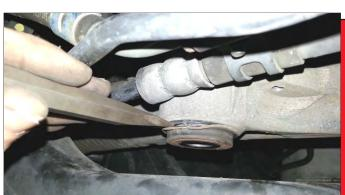
**Passenger side:** The rack will move toward the passenger side and forward just enough to remove the bushing. Use a Tie-Down strap to hold rack in place while removing bushing.
