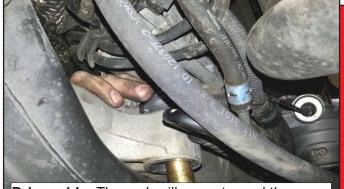
**Driver side:** The rack will move toward the passenger side and forward just enough to remove the bushing.
