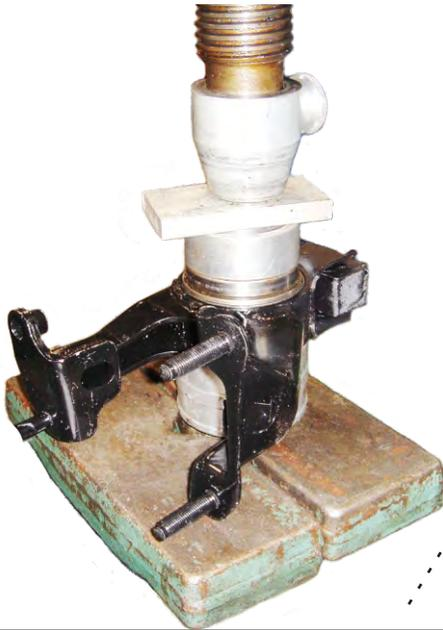
Cut only through this metal shell that is bonded to the rubber mount
