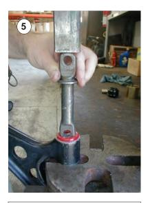
Apply grease to all metal parts that contact the polyurethane bushings. Press in bushing 3335 first, then press the pin in. Don't let the pin push the bushing through other side.
