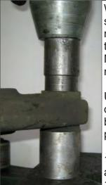
When pressing out bushings and shells, it is good practice to remove and replace one at a time to maintain good rear alignment. Mark cam eccentrics prior to removal to aid in re-alignment.
