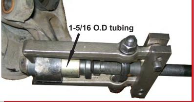
NOTE: ! CHECK SPHERICAL BEARING PRIOR TO PRESSING OUT! IF TIGHT, DO NOT REPLACE
