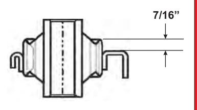
Press the new shell into the control arm until there is 7/16" sticking out on the upper side of the control arm. Install the bushing with p/n 3528 up. Only grease the leading edge to help get the bushing started. Do not grease the I.D. when installing the inner sleeve.
