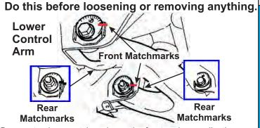
Be sure to place matchmarks on the front and rear adjusting cams before you start. You will need to use these matchmarks to reinstall the lower control arms back in the same position after the new polyurethane bushings are installed. Torque to 100 ft-lbs.
