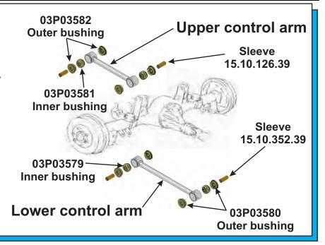
UPPER CONTROL ARMS HAVE NO SHELLS, O.E. BUSHINGS ARE NOT BONDED TO EYE. LOWER CONTROL ARMS HAVE METAL SHELLS AND THE O.E. SHELLS MUST BE PRESSED OUT. When pressing out the outer metal shell of the original bushing, you need to push it with something smaller than the inside diameter of the control arm. And the receiver end needs to be bigger than the outside diameter of the old metal shell being pushed out.
