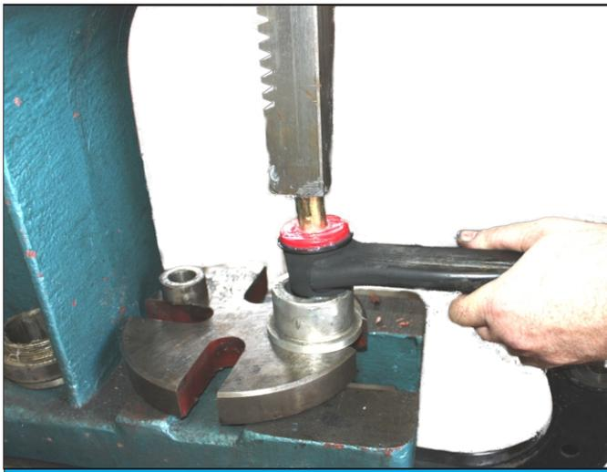
Use a wire brush to remove any remaining old rubber. File off any sharp edges that will contact the new polyurethane bushings. Apply grease to all metal parts that contact the polyurethane bushings. Install upper control arm and through bolts then torque to 60 ft. lbs.
