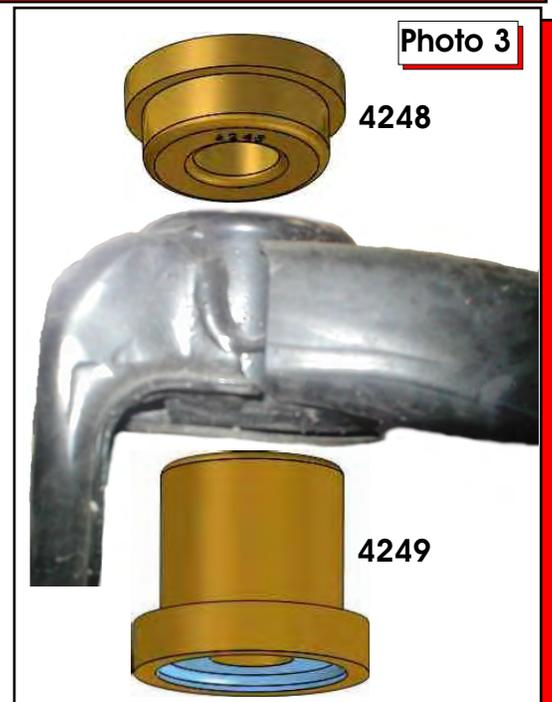
**GREASE ALL PARTS THAT COME INTO CONTACT WITH POLYURETHANE**
